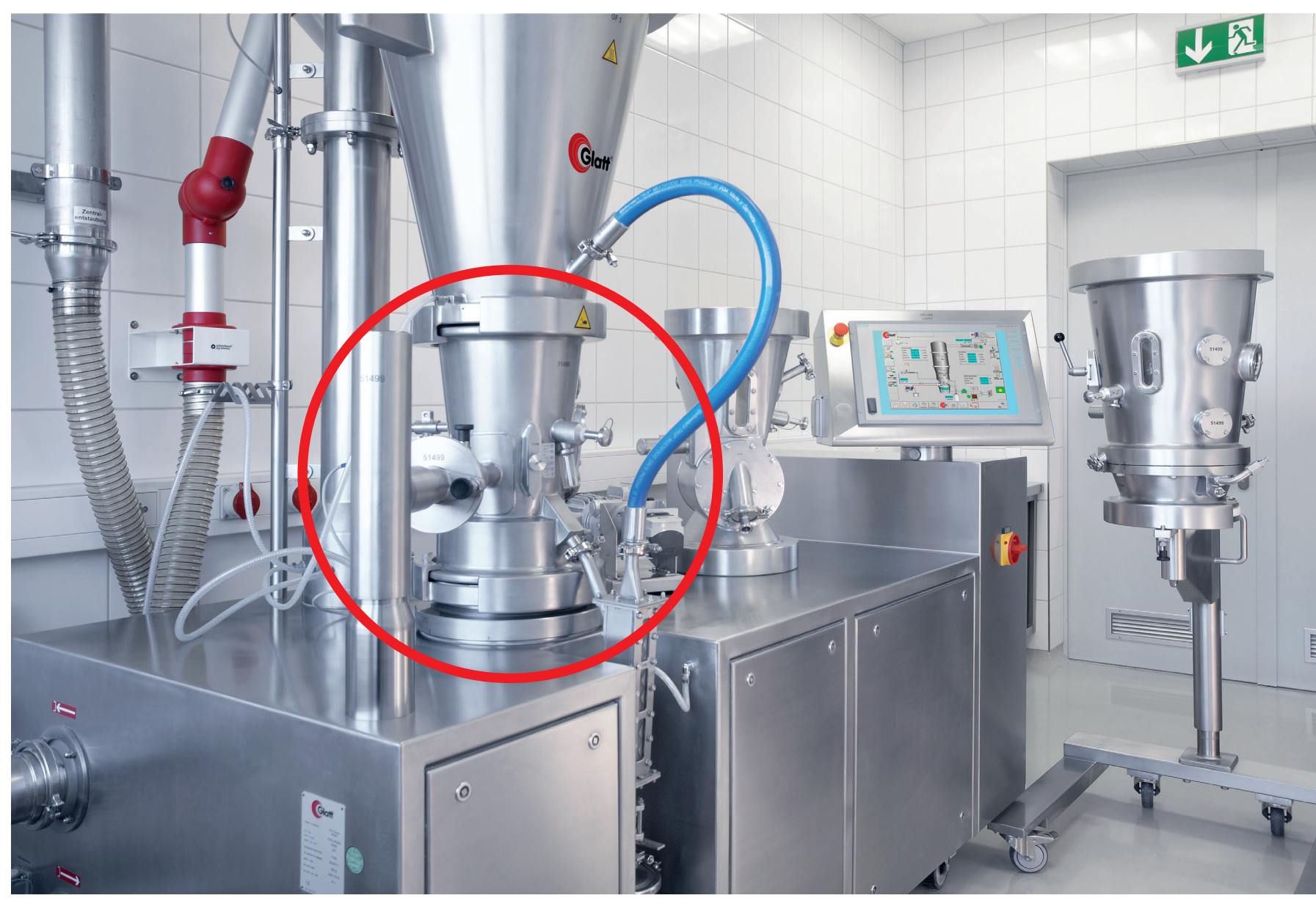
Fig. 1 Application of ultra-thin layers in film coating: The coating material is applied by spraying the solids-containing liquid onto the fluidized particles, and the film is dried and solidified in a single process step. The coating liquid is sprayed onto pre-coated solids. The supplied process air evaporates the liquid and dries the film layer. Small droplets and low viscosity ensure uniform distribution and thus a high-quality film.
