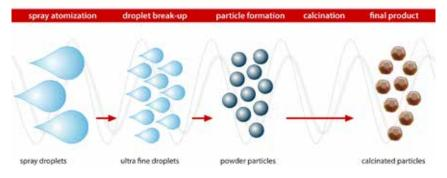
In particle design with Glatt Powder Synthesis, the process steps of particle formation, drying, and calcination can be combined in a single step. All particles undergo the same thermal treatment.
