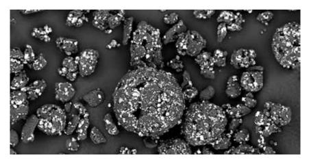
Carbon-silicon anode material
