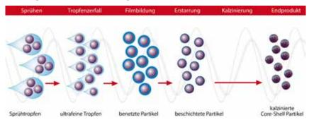
Glatt Powder Synthesis is also used as a process for coating nano- and micrometersized powders. To achieve this, suspensions are used as raw materials. Here, the coating material is dissolved in the liquid phase and is dried onto the core material. If necessary, further thermal post-treatment (e. g. calcination) can be carried out in the same process run. Glatt Powder Synthesis coating processes have the same advantages and thermodynamic conditions as already described.
