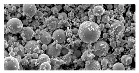
Barium-strontium-cobalt-iron oxide powder for oxygen membranes and for hydrogen synthesis
