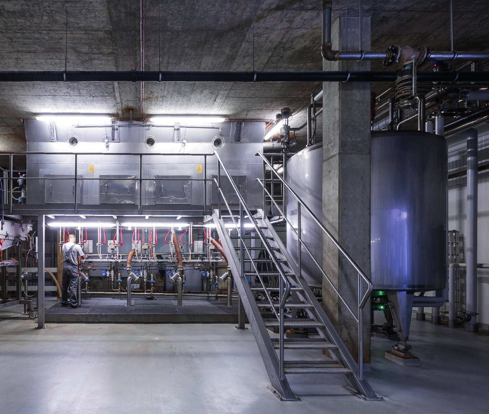
Batch fluid bed processing in circular plant Credit: © Erbo Spraytec
