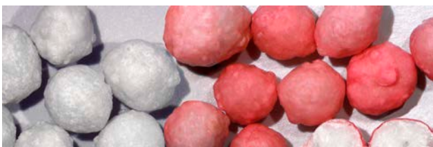
Figure 4. Fertilizer granules before and after coating.
