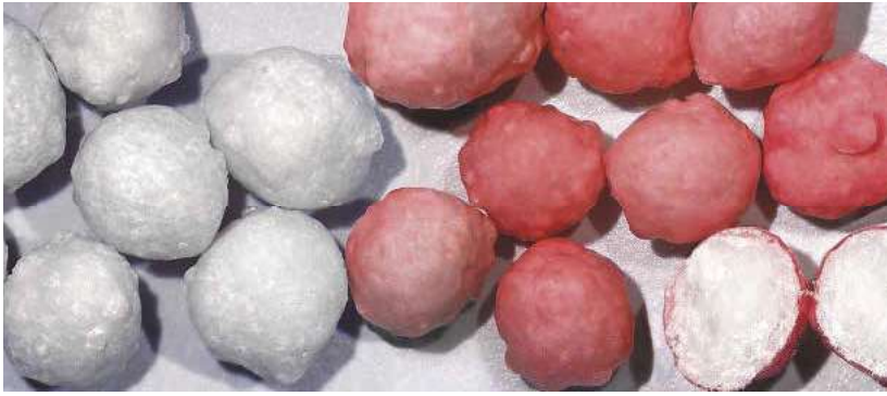
The fertiliser granules can be coated with a coloured branding or with a pH-controlled release profile
