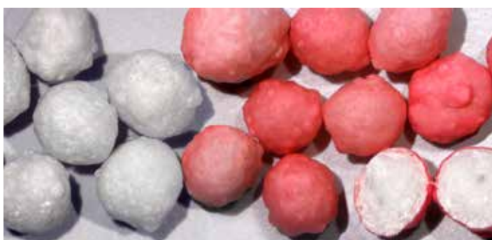
Figure 3. The fertilizer granules can be coated, for example, with a specific colour or a pH-controlled release profile.
