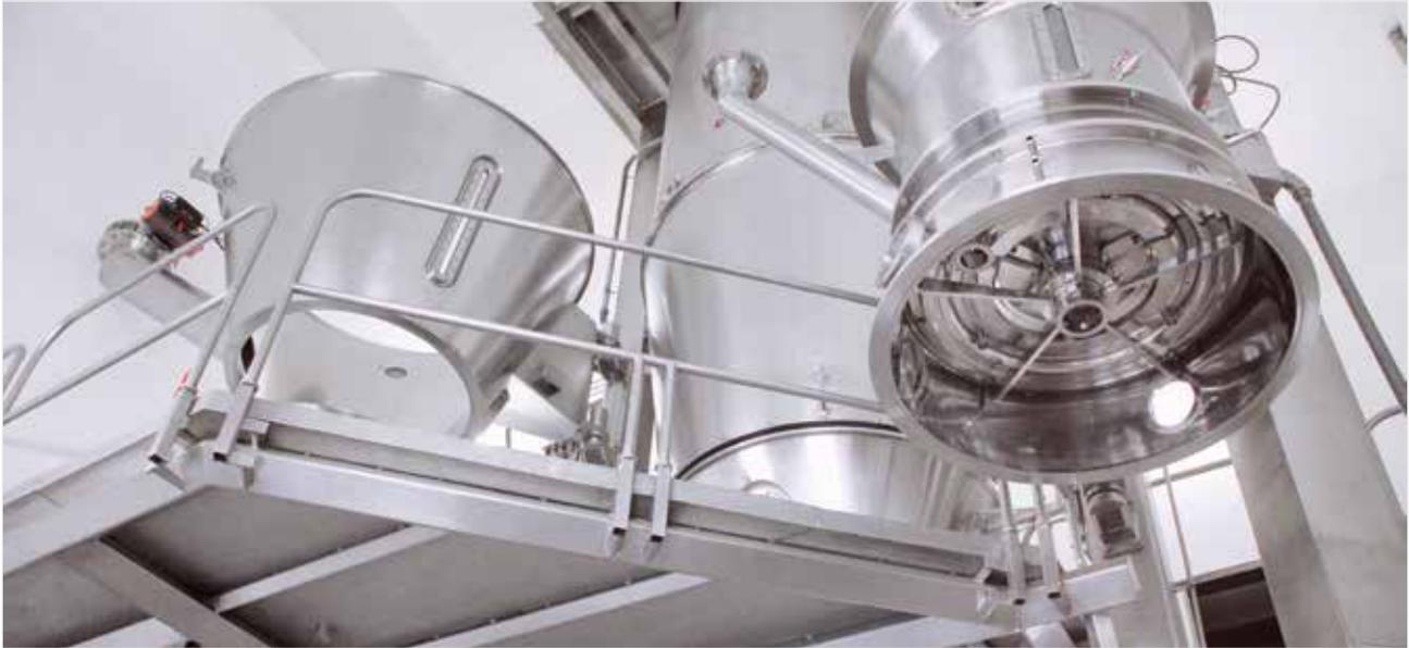
The ProCell series combines the innovative spouted-bed concept with the flexibility and multi-zone concept of a GFG. The main areas of application are the granulation of fine particles, processing of materials that are sensitive to temperature and retention time, and processing of sticky materials.
