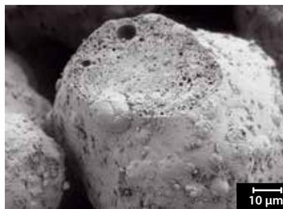
Granule with oil encapsulated in the matrix
